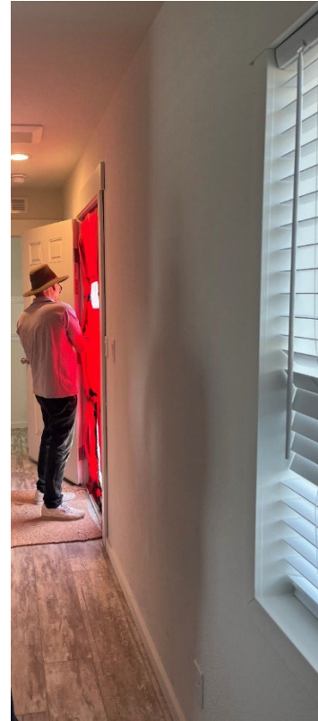
Figure 7: Blower door test at the site. EPRI. 2023.
